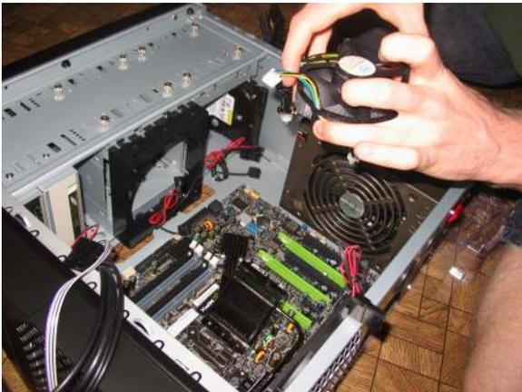
Attach the CPU heat sink.
