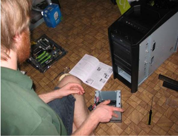
Put the hard drives into their bays, and attach the data cables to the motherboard, and the power cables to the power supply.
